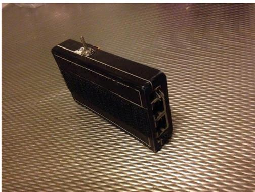
Figure 5. The complete design of the hexaphonic preamp.
